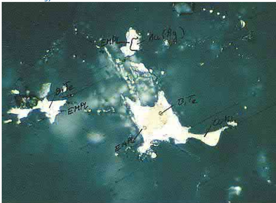
Gold (yellow), emplektite (medium-grey margin) and Bi telluride (pale grey) associated with silicates and chalcopyrite (cuki) at Ängesneva. Field of view 0.026 mm. From Kojonen et al. (1991).
