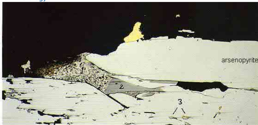
Gold in contact with arsenopyrite. Bi-Te sulphide (1) and tetrahedrite (2) in fractures of arsenopyrite, Bi-telluride (3) as inclusions in arsenopyrite. Ängesneva. Field of view 0.052 mm. From Kojonen et al. (1991).
